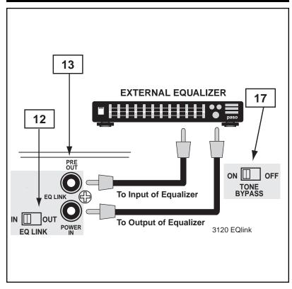
Fig. 20 - Rear Panel External Equalizer Link Diagram
